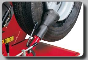
Bead breaking on outside of tyre
