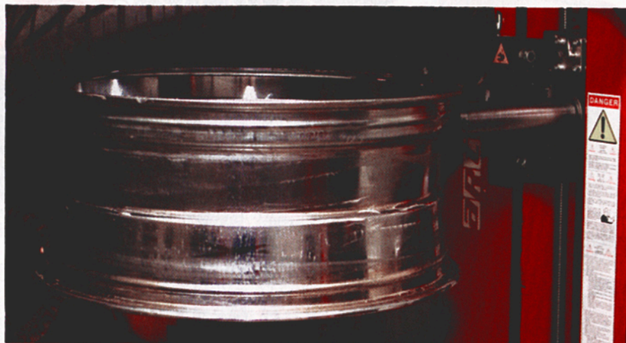
This reverse rim with tire removed shows that the drop area biases to the rear of the wheel. Remember that this wheel is affixed "upside down" on the changer.
