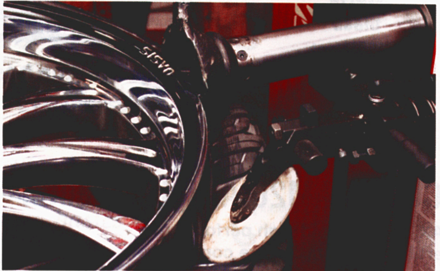
To avoid the use of irons (both for operator safety and to prevent rim or bead damage), machines that feature a roller wheel and a bead controller arm perform all of the hard work while preventing damage.
