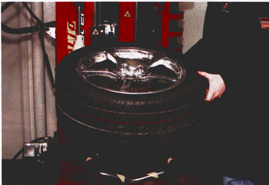
Another problem-child is the run-flat tire, which, because of its extraordinarily stiff sidewall/bead area, can pose a real handling challenge. Here an 18" wheel run-flat package is motored into position.
