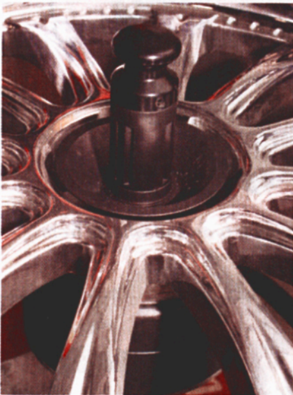
The polymer construction of the cone will not damage the wheel surface.
