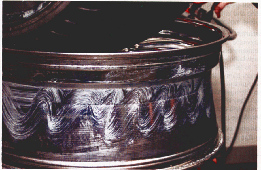
Large diameter (and wide) tires require a bit of mounting lube in the drop center area of the rim to facilitate mounting and bead seating.
