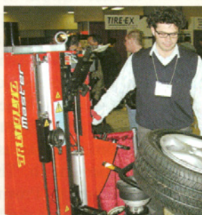
B-Line's Paulo Molinari shows off the Corghi Artiglio Master tire changer that lifts, clamps, breaks the bead, and demounts without touching the rim
